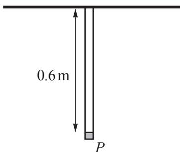
A small object  $P$  is attached to one end of each of two vertical light elastic strings. One string is of natural length  $0.4\text{ m}$  and has modulus of elasticity  $10\text{ N}$ ; the other string is of natural length  $0.5\text{ m}$  and has modulus of elasticity  $12\text{ N}$ . The upper ends of both strings are attached to a fixed horizontal beam and  $P$  hangs in equilibrium  $0.6\text{ m}$  below the beam (see diagram).
