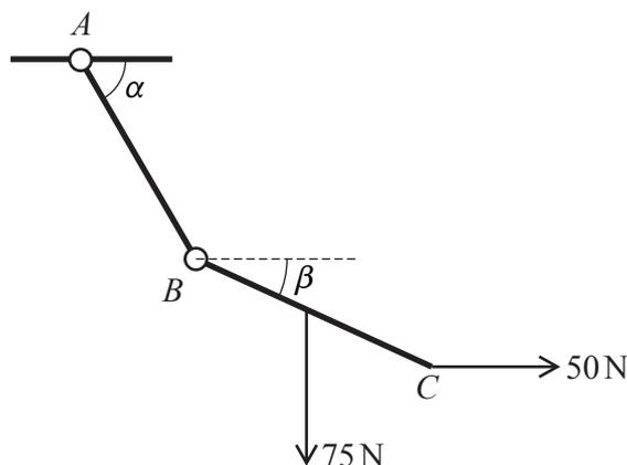
Two uniform rods  $AB$  and  $BC$ , each of length  $2L$ , are freely jointed at  $B$ , and  $AB$  is freely jointed to a fixed point at  $A$ . The rods are held in equilibrium in a vertical plane by a light horizontal string attached at  $C$ . The rods  $AB$  and  $BC$  make angles  $\alpha$  and  $\beta$  to the horizontal respectively. The weight of rod  $BC$  is  $75\text{ N}$ , and the tension in the string is  $50\text{ N}$  (see diagram).
